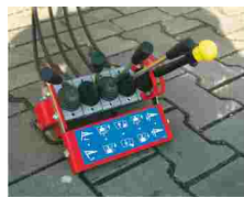
Remote control by bowdencable operation.
