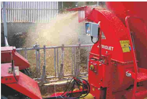
Distribution width strawbedder: 15-18 m.
