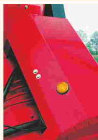
A monitoring light indicates that feed has been cut out right to the bottom of the clamp.
